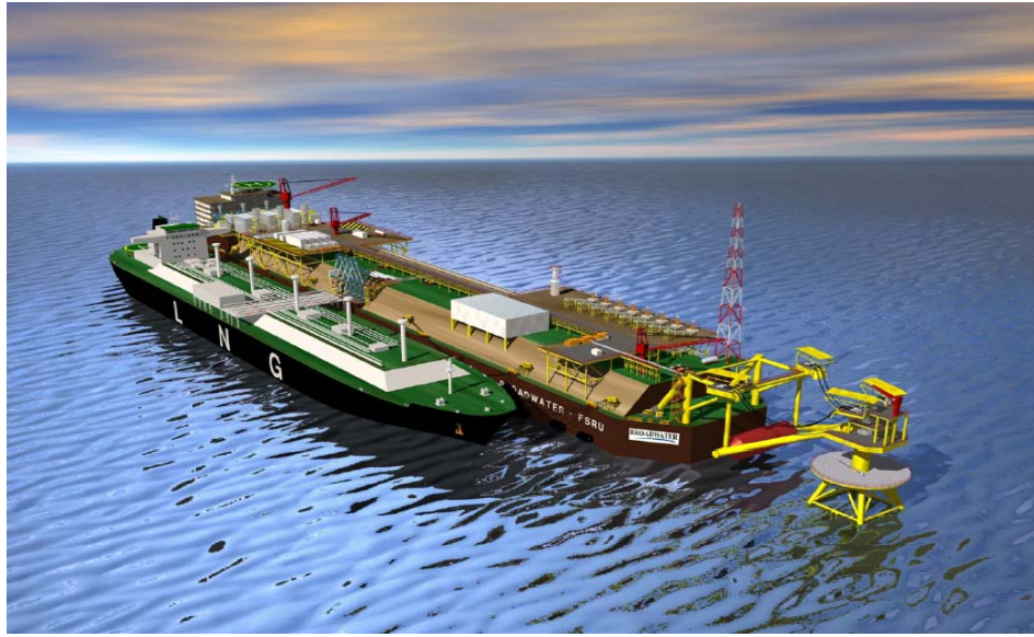
Figure 37 – FSRU with Moored LNG Carrier 99
